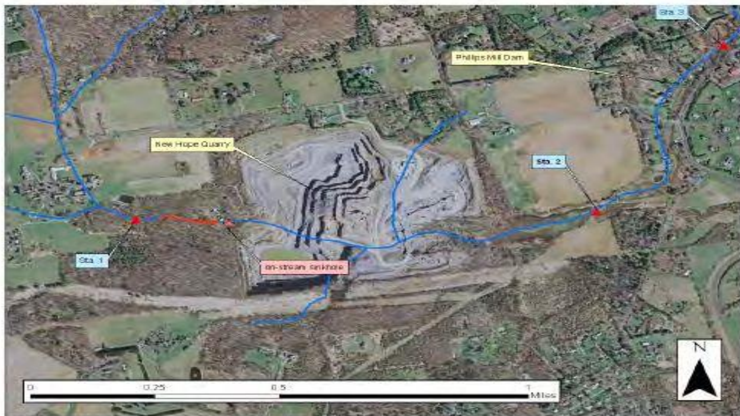
Figure 1. 2005 DVRPC Aerial Photography showing Primrose Creek Watershed in proximity to New Hope Crushed Stone quarry. Survey stations shown as red triangles, On-stream sinkhole shown as pink asterisk, channel head-cut shown as red line.
