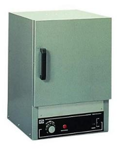
Determine conditions to dry filter/sample to constant weight at 105 C Aluminum weighing dish/boat recommended (also on Amazon)
