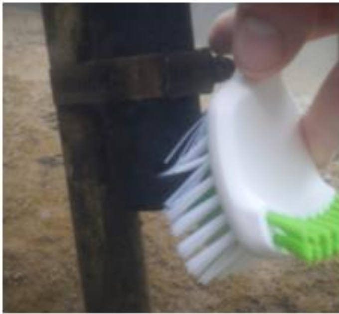
Photo 6. Cleaning the screw heads inside the CTD sensor.
