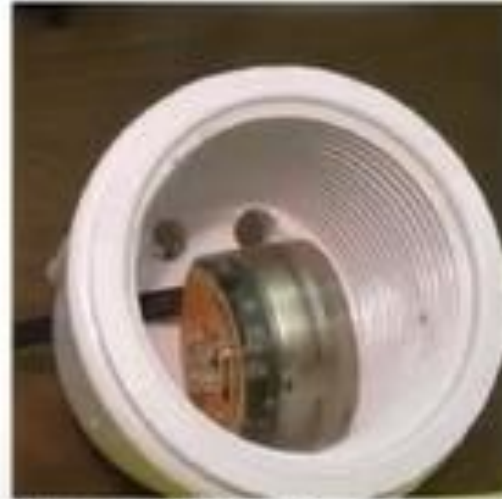
FIGURE 7. TIDBIT FASTENED INTO PVC CAP USING A TIE STRAP (ZIP TIE).
