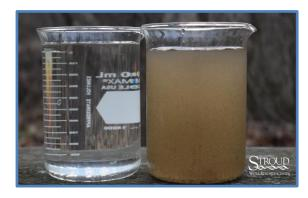
sending a beam of "near-infrared" light into the stream and measuring how much light is reflected back into the sensor. If more light reflects back, then the meter reads the water as more cloudy. Less light will reflect back when the water is clear.
