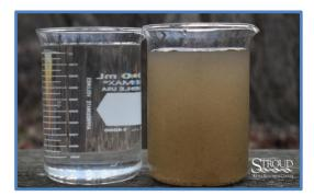
stream and measuring how much light is reflected back into the sensor. If more light reflects back, then the meter reads the water as more cloudy. Less light will reflect back when the water is clear.
